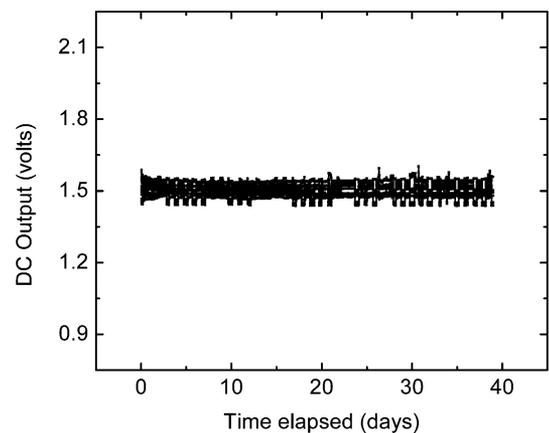
Fig. 8. Typical life test data for a silicone (NuSil 2188) encapsulated assembly. Life tests monitor the output of a device immersed in  $0.9\%$  saline solution at room temperature. Steps in the data are due to light sensitivity.
