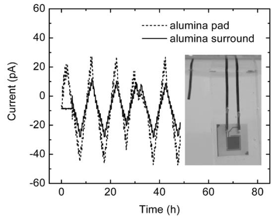
Fig. 7. Representative data from encapsulation current leakage tests (reference electrode driven, guard ring at ground). Inset: an alumina substrate with gold conductors encapsulated in silicone in  $0.9\%$  saline solution. The other wire is a platinum reference electrode.
