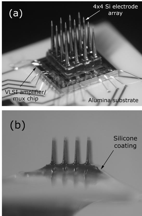
Fig. 2. Electrode and amplifier assembly (a) prior to and (b) after silicone encapsulation.
