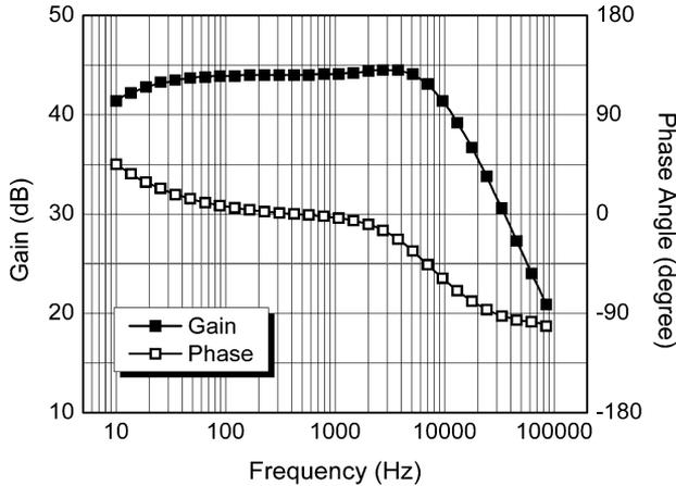
Fig. 1. Bode plot of the response of one channel of the amplifier IC.
