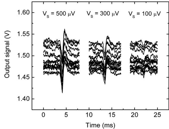
Fig. 3. Amplifier output for the pseudospike excitation in ACSF solution, showing detection capability of the hybrid neuroport. Raw data with various amplitude pseudospike suggests the system detection limit below 100  $\mu\text{V}$ .
